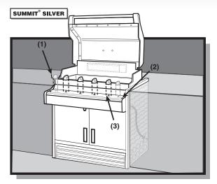
Put your fingers under the front edge of the control panel and lift off.
